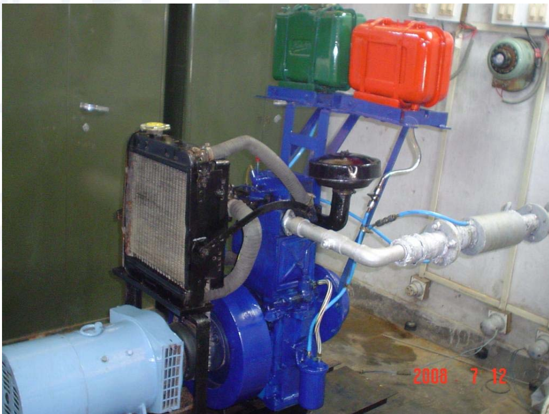
Engine Setup for Using SVO as Fuel
