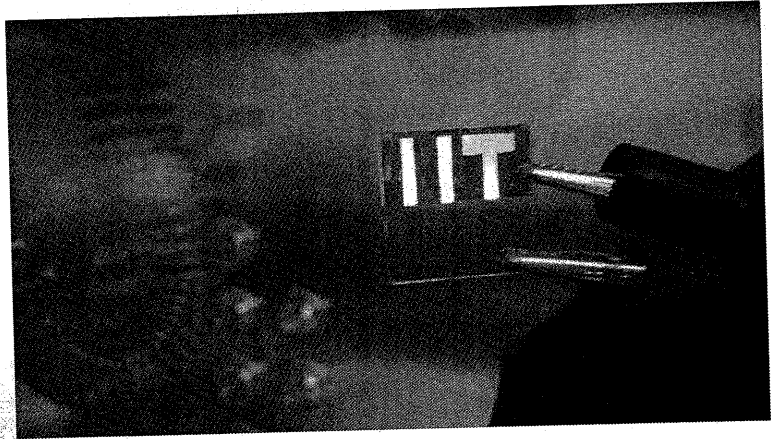
Figure 5: PF-DPA polymer OLED device operating in a glove box
