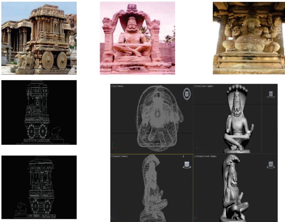
Hampi monuments, 3d laser scanned images, cad diagrams generated from terrestrial laser scanned point cloud data
