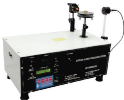
Developed SPR measurement system utilizing a precision rotation stage
