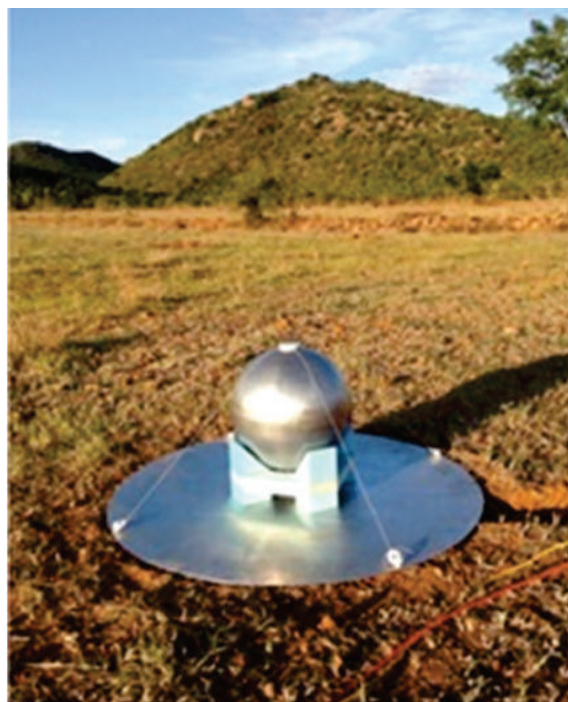
A precision radiometer called SARAS 2, built at the Raman Research Institute deployed in a radio quiet site in Timbactu Collective in Andhra Pradesh
