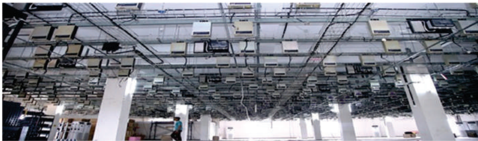
The 619-element antenna arrangement of ST radar at CUSAT
