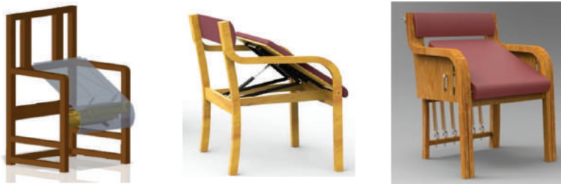
Compliant Easy Chair with features of Bistability and Static Balancing
