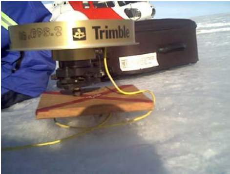
Figure 11: Monumentation on the Schirmacher Glacier in Antarctica
