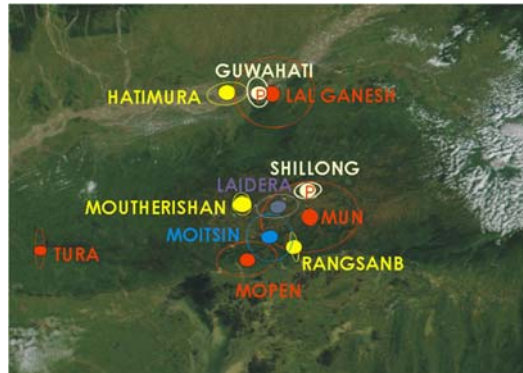
Figure 17: Location of points currently occupied in the Shillong Plateau with the uncertainties in their position. The stations marked in white are permanent stations.
