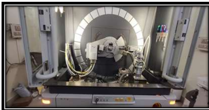
Fig. Powder X Ray Diffraction facility of SAIF at Gauhati University, Guwahati
