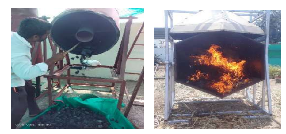
Fig. Charcoal Kiln for loose biomass, capacity 200 kg by ARTI Pune
