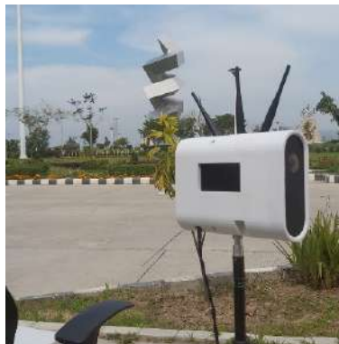
Fig. Picture of Digital Entomologist ( Biodiversity sensor)
