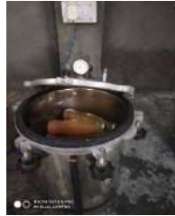
Fig. Retorting at 15 psi for 15 min by STD
