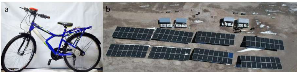
Fig. a) Rapidly charging E-cycle b) Solar photovoltaic array and VRFB system.
