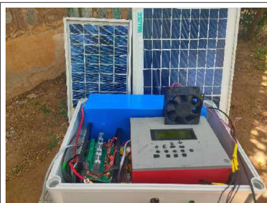
Fig. IoT solar dryer controller prototype by Barefoot College, Tilonia, Rajasthan
