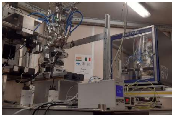
Fig. Experimental Station with HP-HT set-up installed on the sample stage (allowing diffraction measurements up to 30 GPa and 1000 K)
