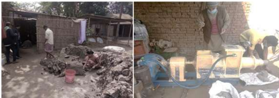
Fig. Existing manual clay processing vs. use of de-airing pug mill
