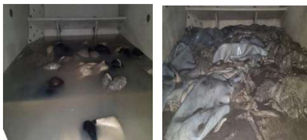
Fig. (a) Cow hides flooded with 100% water in the drum (b) Cow limed pelts after 24 hr of treatment with 100% water, 2% lime and 2% sodium sulphide showing the complete hair removal at M/s Flamingo SSI, Ranipet
