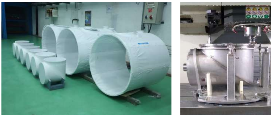
Fig. Service module, Jumper Vacuum Vessel (L), Jumper vessel machining (R)
