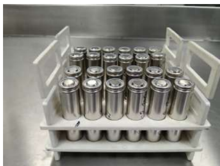
Fig. Li-ion Cells Fabricated using indigenously developed carbon coated LFP
