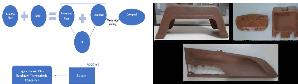
Fig. Steps involved in preparing Lignocellulosic Fiber Reinforced Thermoplastic Composites and High-end prototypes developed from natural fiber PP composites
