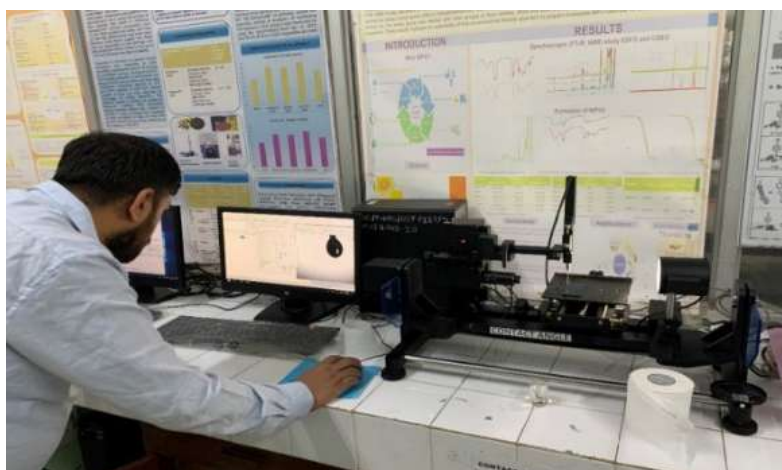
Fig. Contact Angle System Measurement at ICT, Mumbai
