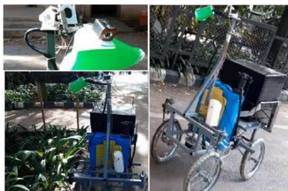
Fig. Agrobot for Plant Disease Analysis and Control
