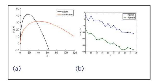
Figure 3 (a) Variation of free-energy of cluster of Orcinol for two different polymorphs in nitromethane. The figure shows that the metastable form has lower free-energy barrier to nucleation and hence is preferentially formed upon crystallization. (b) Free-energy of isolated clusters of Orcinol of various sizes for two different polymorphs
