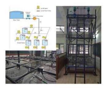
Fig. 9. Clockwise from top left -- Schematic of sub-network, Fabricated experimental facility and Distribution network equipped with necessary instruments.
