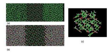
Figure 2 (a) Slab of Orcinol crystal immersed in chloroform. Setup used to compute Orcinol-Chloroform interfacial tension (b) Slab of Orcinol crystal immersed in nitromethane. Setup used to compute Orcinol-Nitromethane interfacial tension (c) Crystalline cluster of Orcinol in vacuum. Setup used to compute free-energy of the cluster
