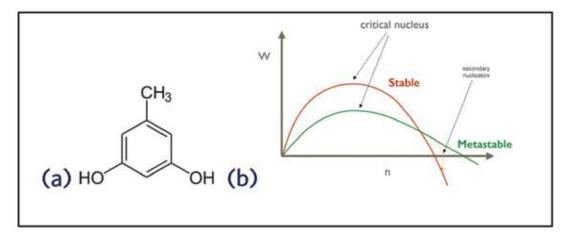
Figure 1(a) Molecular structure of Orcinol (b) Profile for free-energy of formation of nuclei of a stable and a metastable crystal polymorphs during crystal nucleation from a solvent
