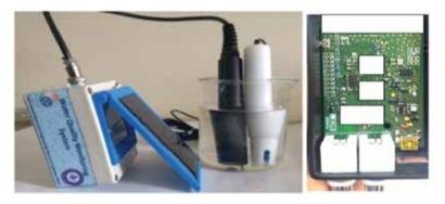
Figure 8. Handheld battery operated smart water quality measuring device developed by the CSIR-CEERI
