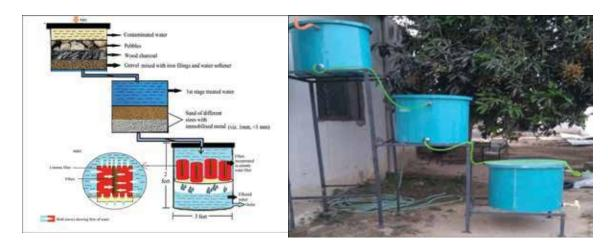
Schematic diagram of the integrated water filter system
