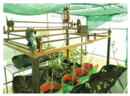
Fig. Automatic fertilizer supply system
