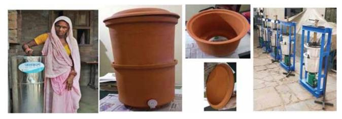
Figure. 5. Biosand Filter Technology (Jalkalp) for removing biological contamination and iron deployed in state of Bihar
