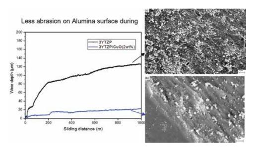
Figure - 2: Left plot indicate the resistance to wear of the Alumina, Right top – indicate the rough worn out surface without addition of CuO, Right bottom - with CuO surface is retained and wear is low. Source: ASME Journal of Tribology (2019)
