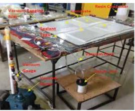
In-house developed VARTM setupIn-house developed wind turbine blade
