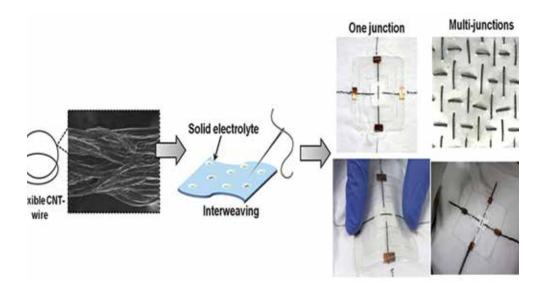
Figure 3. Carbon nanotube coated cotton yarns that are used in wearable electronics.
