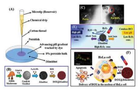
Figure – 4 (A-F) shows the process flow of FeNP nanobot synthesis, micrograph of FeONP, drug loading, mechanism of moving using magnet and delivery of attach drug to a specific site in the cell cluster. Source: ACS Biomaterials Science & Engineering, 3, 1627 (2017)
