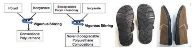
Polyurethane foaming process
