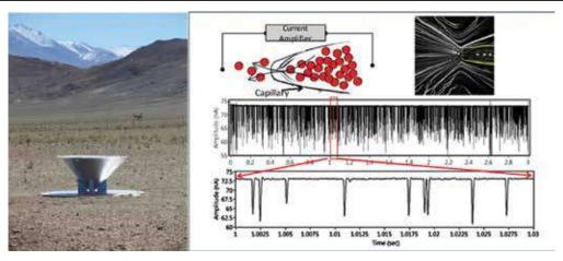
(Left) Precision Radiometer SARAS 3 deployed at IAO, Hanle, a site operated by the Indian Institute of Astrophysics. (Right) Electro-fluidic device for measuring cellular morphology changes as early biomarkers of disease. Top panel shows time integrated image of fluidic field lines of model cells translocating through the micro-orifice. Bottom panel shows the corresponding electrical signature that is used to relate the cell morphology to the cell state.
